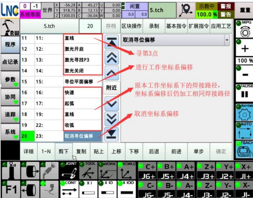
This function is a three-point plane positioning, which is limited to use when the workpiece needs two adjacent right-angled edges. Based on this, an improvement has been made to calculate the accurate offset by finding four points. The method is as follows:
