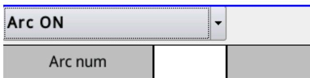
Arc starting:  , added at the arc starting point, outputting an arc starting signal to the welding machine, and can set the welding arc number (corresponds to the group number in the parameter page-arc welding page-arc welding sequence page)
