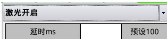
: Turn on the laser and tracker. You can set the delay time after turning on, the preset is 100ms.
